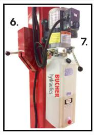
Energy efficient US Made Bucher 2HP / 1.5kw power unit typically lasts the life of the lift - single point lock release - rubber motor mounts
