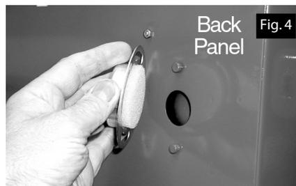
Insert the circular foam filter into the recess in the Air Vent Cover, and attach the cover to the rear of the cabinet as shown in Fig.4, having first pried out the plastic bung from the vent hole.
