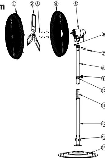
**Note:** Not all components of the 30" Oscillating Pedestal Fan are replacement items, but are illustrated as a convenient reference for location and position in the assembly sequence.
