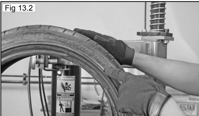
3. Lubricate both tire beads liberally with tire manufacturer's approved lubricant. (See Fig 13.3)
