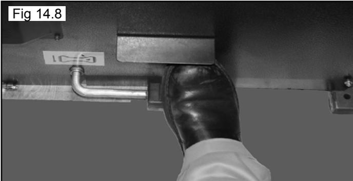
**TO SEAL LOW PROFILE OR DIFFICULT BEADS, USE THE TURBO BLAST TO SEAL THE BEAD**
