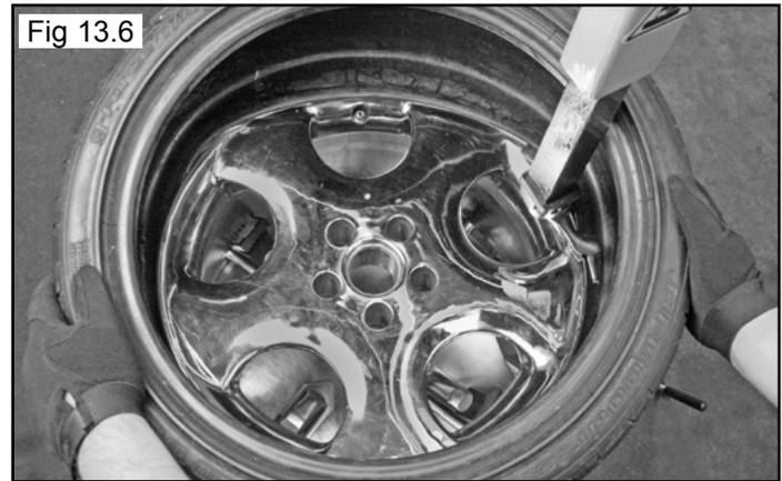
6. For the top bead, rotate the Table Top until the valve stem is at the 3 o'clock position in relation to the Mount/ Demount Head. Lift the upper bead above the right side of the Mount/ Demount Head and below the knob. (See Fig 13.7)
