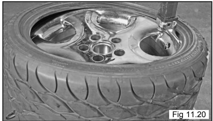
12. Liberally lubricate the lower bead again, if there was any difficulty lubricating the lower bead earlier. (See Fig 11.21)
