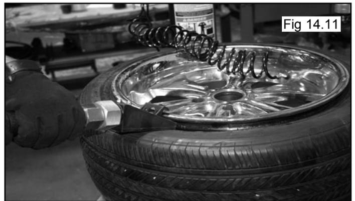
4. Depress inflation pedal and open the Turbo-Blast Valve for less than one full second. The blast of air from the Turbo Blast Nozzle will expand tire and seal the beads.
