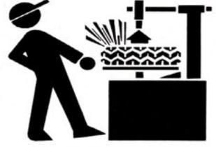
**STAND CLEAR WHILE INFLATING TIRE. TIRE OR WHEEL FAILURE UNDER PRESSURE MAY CAUSE SERIOUS INJURY OR DEATH.**
