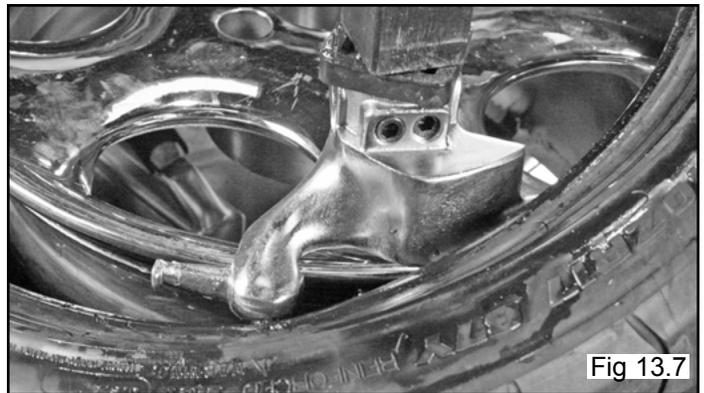
7. With the Bead Lifting Tool, press down on the tire to hold the upper bead in the drop center. (See Fig. 13.8)
