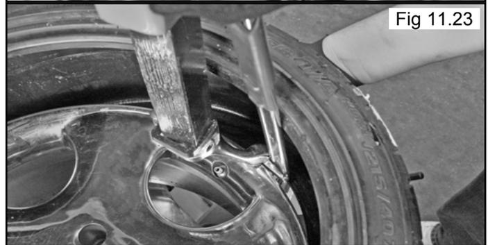
15. Depress the Table Top Pedal to rotate the wheel.
