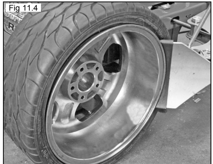
8. Determine the mounting side of the wheel. The mounting side is the narrow side of the drop center. (See Fig. 11.5 on page 16)
