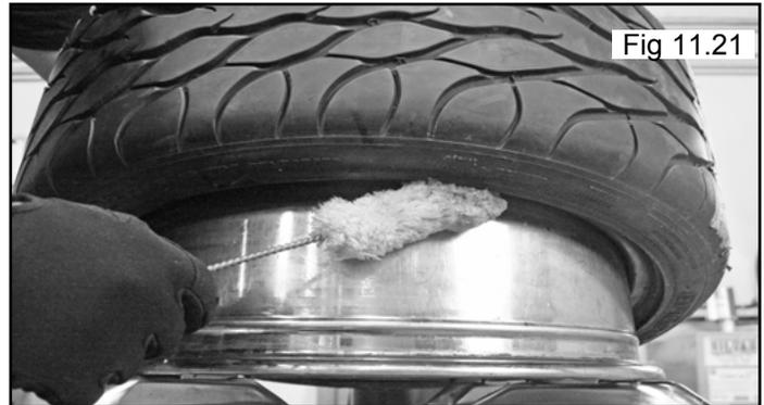
13. Lift and hold the tire so it is positioned with the lower bead in the drop-center portion of the wheel.
