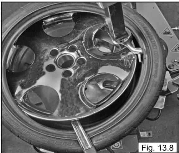
8. Stand firmly in place and be prepared to hold the Bead Lifting Tool down as the tire/ Turntable rotates. Depress the Table Top Pedal and rotate the tire until the bead is mounted. (See Fig. 13.9 - 13.12)
