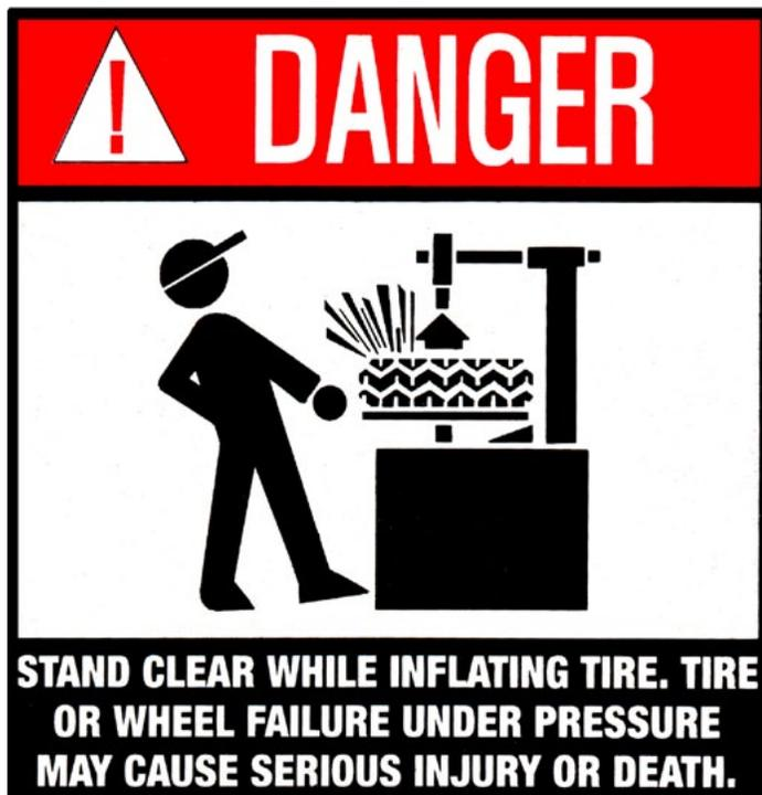
1. Once tire pressure is indicated on the pressure gauge continue to inject air into the tire in short intervals. Check the pressure frequently. Stand back during bead seat. Keep hands, arms, and entire body away from tire during this procedure. Tire beads should move outward and “pop” into their bead seat position as pressure inside the tire increases. If this does not happen, a problem exists. Investigate carefully. (See Fig 14.12)
