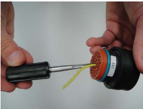
1. With rear insert toward you, snap appropriate size extractor tool over the wire of contact to be removed
