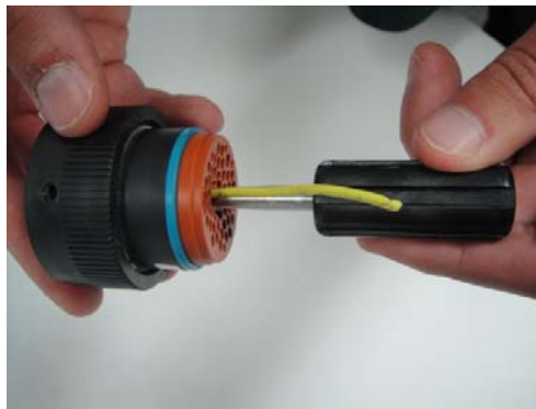
2. Slide tool along into the insert cavity until it engages contact & resistance is felt.
